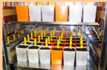
Experiment to determine the effect of A. bisporus on prochloraz degradation in a controlled environment cabinet
